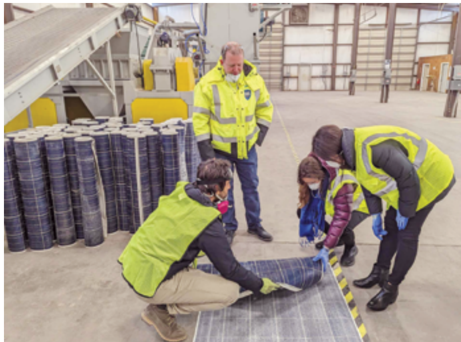
SOLARCYCLE's CTO, Pablo Dias and COO, Rob Vinje, showing laminate after it has been cleanly separated from the glass to investors and partners. Laminate is where most of the value is contained in a panel, as in silver, silicon, and copper. (Solarcycle)
