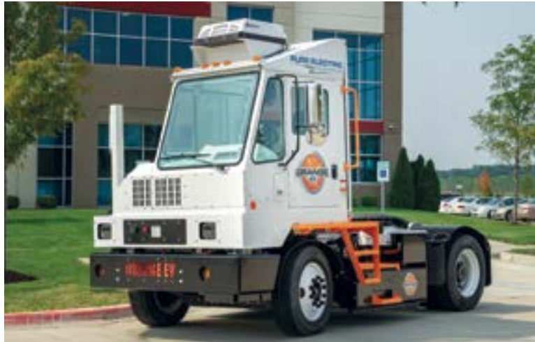
EV yard trucks are used by Ben and Jerry's for loading product. This will eliminate 90 tons of carbon emissions and 9,000 gallons in diesel fuel per year. (Orange EV).
