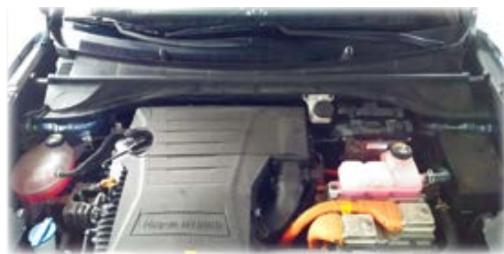
The engine compartment includes the internal combustion engine, transmission, and electric motor and the windshield washer fluid filler- bottom left!
