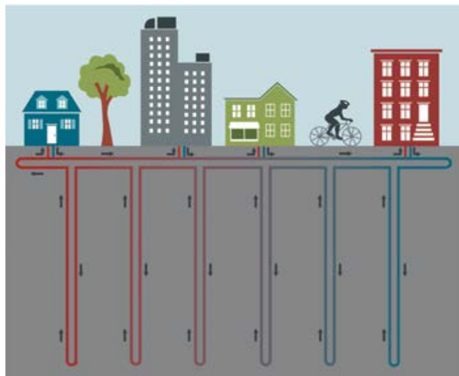
Networked geothermal moves heat into and out of buildings. The primary source of heat is the ambient temperature underground, though the systems also transfer “waste” heat between buildings with different heating and cooling needs, increasing efficiency. (HEET)
