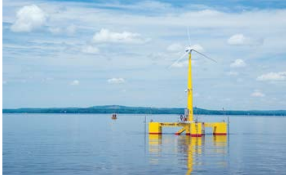
University of Maine's 20-kilowatt grid-tied offshore wind turbine in a 2013 demonstration off Castine, Maine. (Jplourde umaine, CC-BY-SA 4.0, https://bit.ly/CC-by-SA-4-0 )
