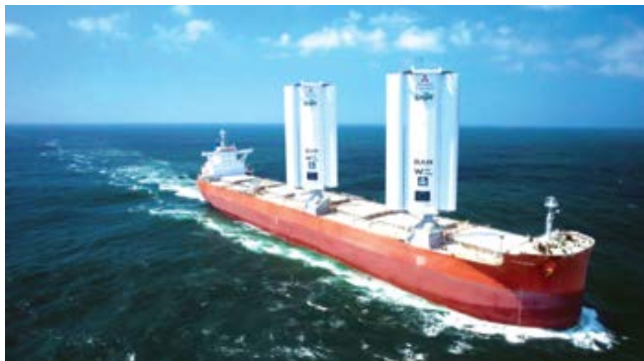
The 2017 Mitsubishi bulk cargo ship Pyxis Ocean , chartered by Cargill, was retrofitted with two of UK's BAR Technologies WindWings. The wing-like sails are estimated to save up to 30% of fuel usage and greenhouse gas (GHG) emissions. (Cargill)
