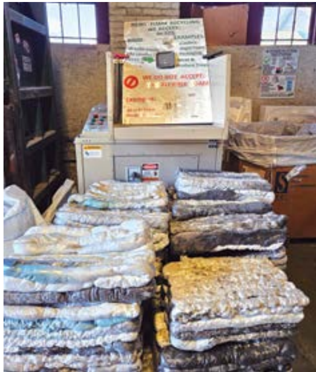
Northeast Kingdom Waste Management District (NEKWMD) purchased a polystyrene recycling machine with grant funding. The machine condenses the material into ignots which will be sold for use in making foam insulation panels. (NEKWMD)
