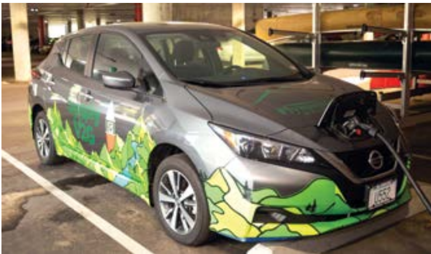
Two Nissan LEAF EVs at PSU provided 1 MWh of energy to the ALLWell Center, offsetting some of the building's electricity needs. Bidirectional EVs, such as the Nissan Leafs' are valuable assets that can help stabilize the grid by dispatching energy stored in batteries when and where that energy is needed most. (Plymouth State University)
